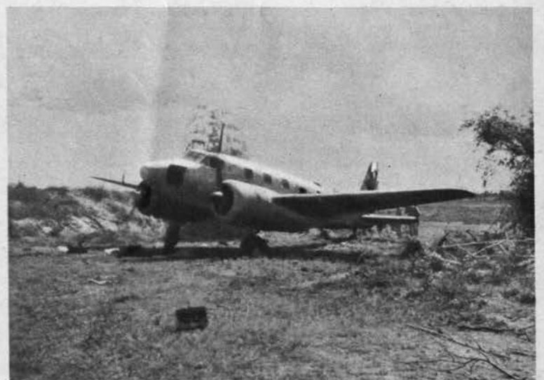
Hickory is twin-engine transport and advance trainer. It is smaller than Helen and Peggy, fatter and slower than twin-engine fighters.
